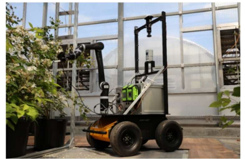
Figure 1: The BrambleBee, one version of a vehicle-mounted pollinator developed by a research group at West Virginia University (Image Credits: Design of an Autonomous Precision Pollination Robot )
